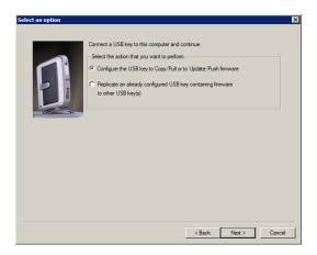
3. Select the Configure the USB key to Copy/Pull or to Update/Push firmware option, and then click Next to open the Select the Configuration dialog box.
